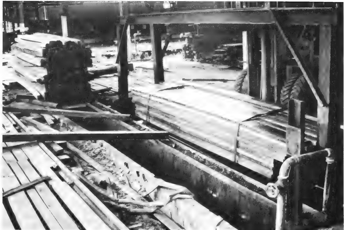
Hardwood lumber being treated with borates using the dip-diffusion method.
